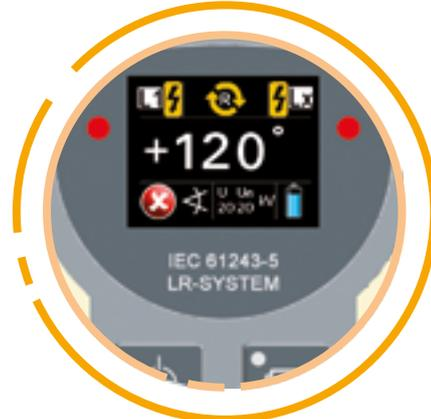
Precise phase angle measurement with phase rotation indicator
