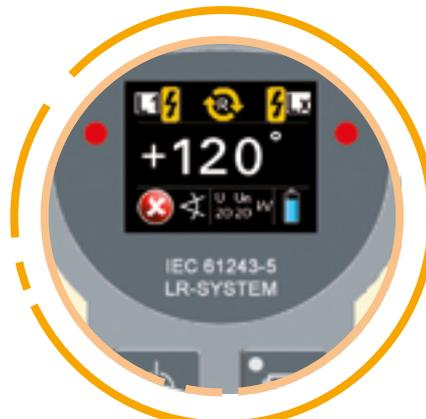
Precise phase angle measurement
